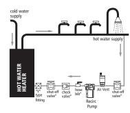
Figures 1,2,3, and 4 are for single line returns only. For multiple branched supply line installations, a recirculation line should be installed for each branch.
