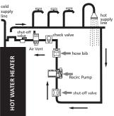
B. Return to Drain Valve at Bottom of Water Heater fig. 4
